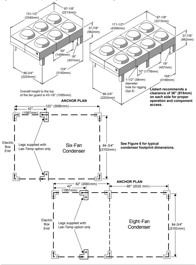
Figure 5 Condenser planning dimensional data—Six- and eight-fan units
